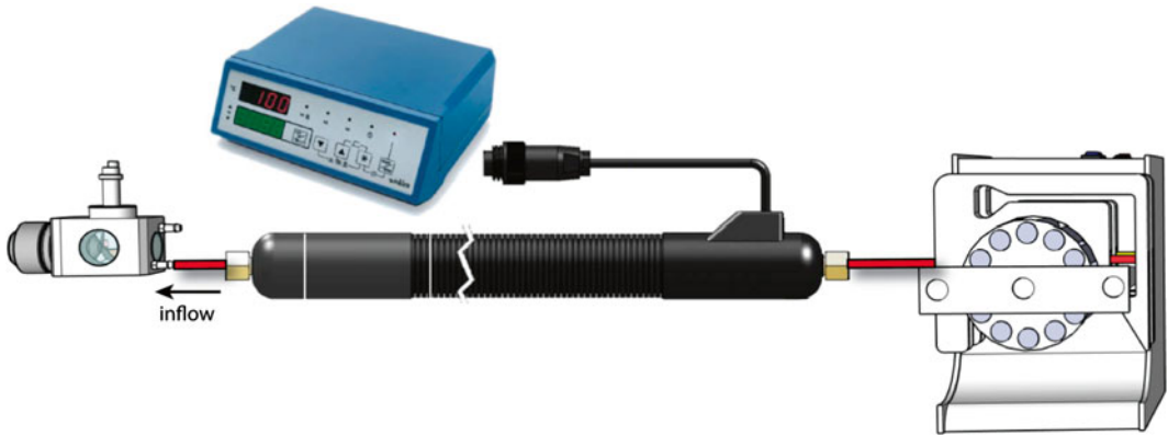
Fig. 8 Assembly of the temperature-controlled heating system. The final part of the inlet tube is inserted through the heating system, which warms the perfused medium
