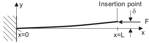
Figure 9.2 Buckling model of a microneedle.
